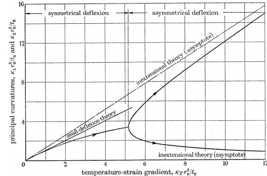
Variation of principal curvatures with temperature gradient through thickness for a lenticular disk.
