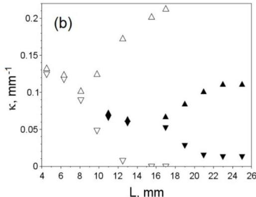
Maximum and minimum curvatures of two square bilayer films with layers in each of approximately equal thickness.
